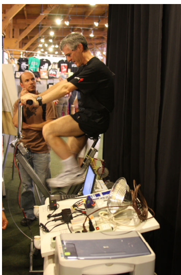
Above: a bicyclist powers common electronic items by pedaling his modified stationary bicycle.
